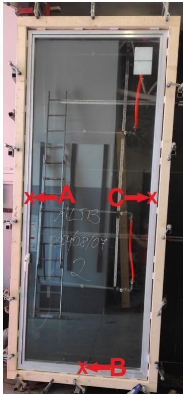
Spacing of measurement points.
